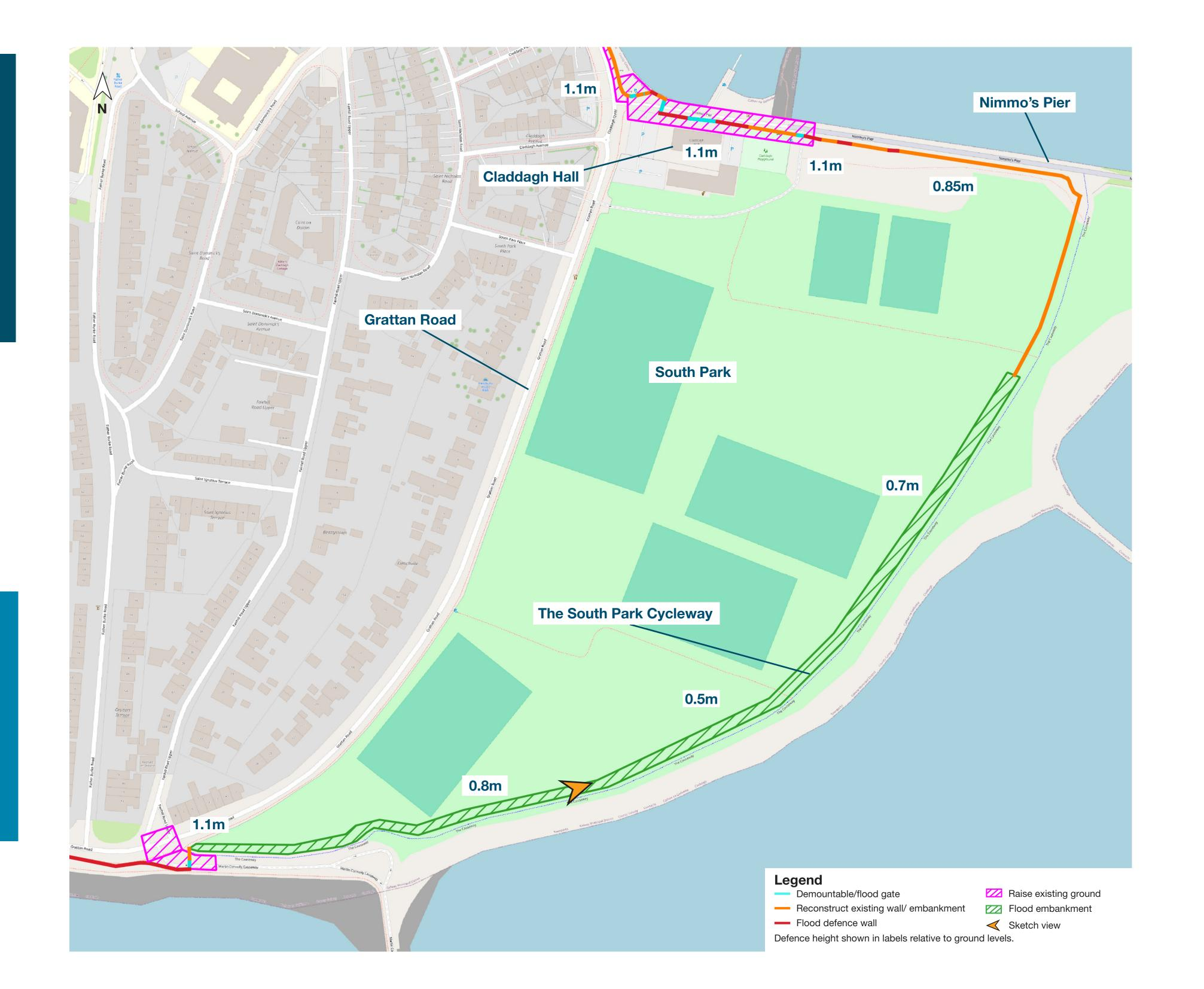
This option consists mainly of raising the South Park cycleway, and maintaining the existing cycle/ walk way. The layout for this option is similar to the one presented in Option 1. The only distinction is that, rather than an embankment positioned behind the South Park cycleway as in Option 1, it is proposed to elevate the South Park cycleway itself to function as the flood defence. Demountables/ flood gates will allow for access to Mutton Island to be maintained.
