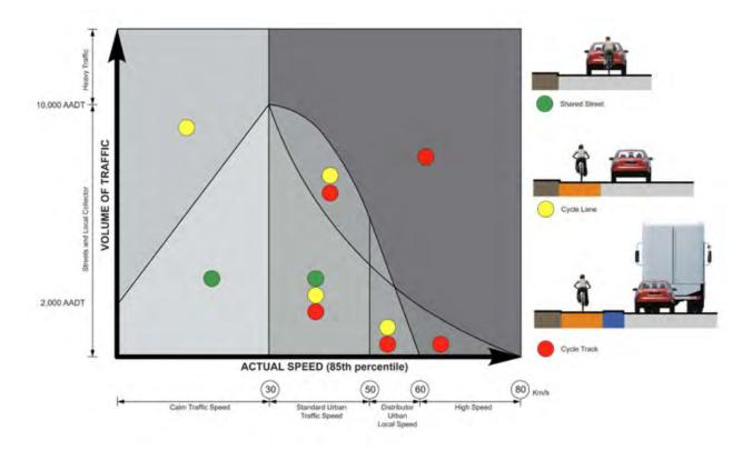
Figure 2.2 - NCM "Mixed or Separate" Calculator
