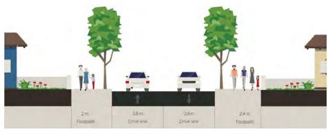
Figure 6.64 - Route 8, Cross Section A-A Existing
