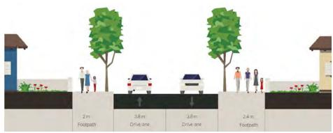
Figure 6.62 - Route 8, Cross Section A-A Existing
