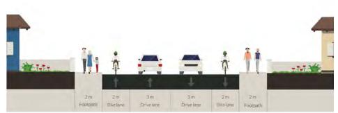
Figure 6.56 - Route 7C, Cross Section A-A Proposed
