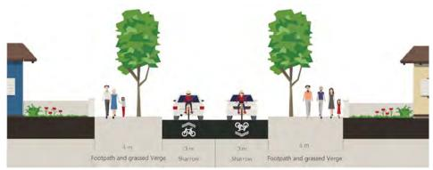
Figure 6.41 - Route 6A, Cross Section A-A Proposed
