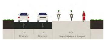
Figure 6.17 - Route 3B, Cross Section A-A Proposed
