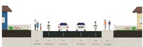
Figure 6.65 - Route 8C, Cross Section A-A Proposed
