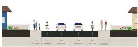
Figure 6.47 - Route 6C, Cross Section A-A Proposed
