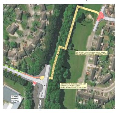
Figure 10.5 - Concept Design of Junction Layout and Ramp from Lucan Road to Sarsfield Park
