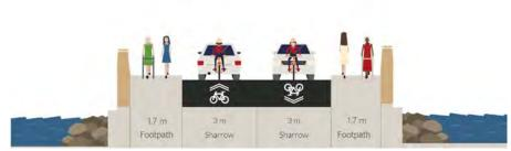
Figure 8.13 - Route 11 A, Cross Section A-A Proposed
