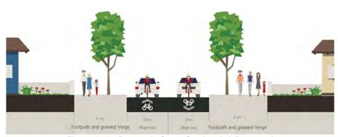
Figure 6.50 - Route 7A, Cross Section A-A Proposed
