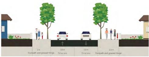
Figure 6.40 - Route 6, Cross Section A-A Existing
