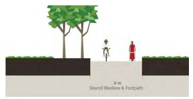
Figure 5.4 - Route 1A, Cross Section A-A Proposed
