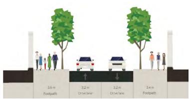
Figure 8.5 - Route 9, Cross Section A-A Existing
