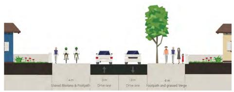
Figure 6.54 - Route 7B, Cross Section A-A Proposed
