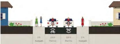
Figure 6.33 - Route 5A, 5B, & 5C Cross Section B-B Proposed
