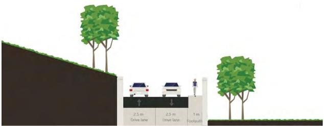
Figure 6.6 - Route 2, Cross Section B-B Existing
