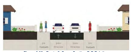
Figure 6.32 - Route 5, Cross Section B-B Existing
