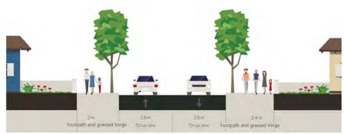
Figure 6.44 - Route 6, Cross Section A-A Existing
