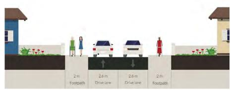
Figure 6.42 - Route 6, Cross Section B-B Existing
