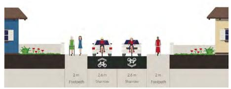
Figure 6.43 - Route 6A, 6B & 6C Cross Section B-B Proposed
