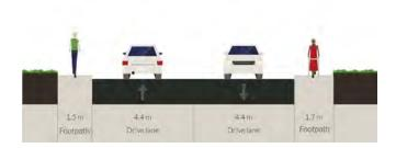
Figure 6.26 - Route 4, Cross Section A-A Existing
