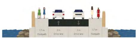
Figure 8.14 - Route 11, Cross Section A-A Existing
