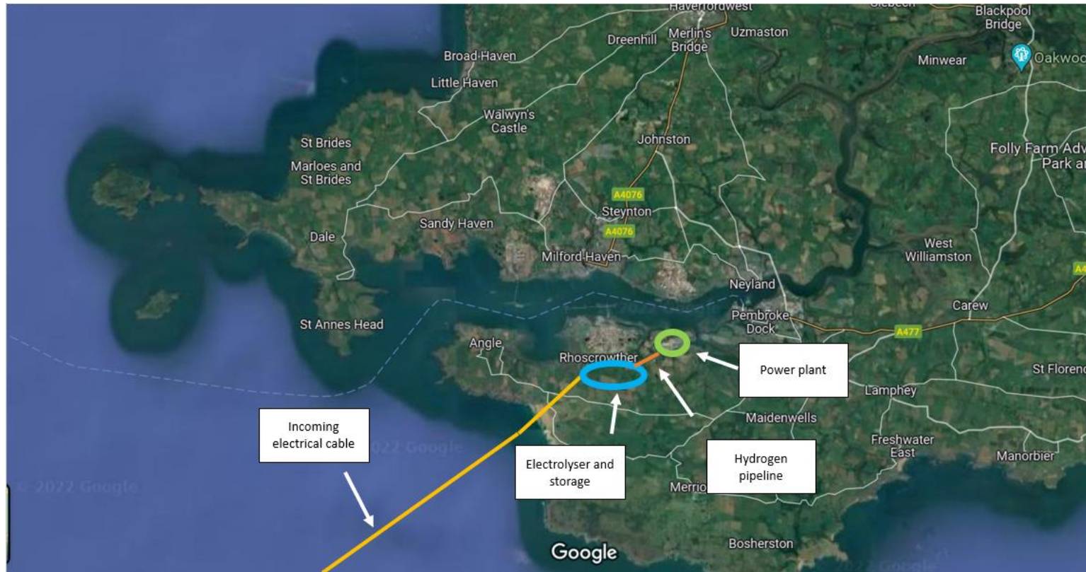
Figure A13: one possibility for landing energy in Option 2 - an electrical cable connected to an electrolyser with storage.
