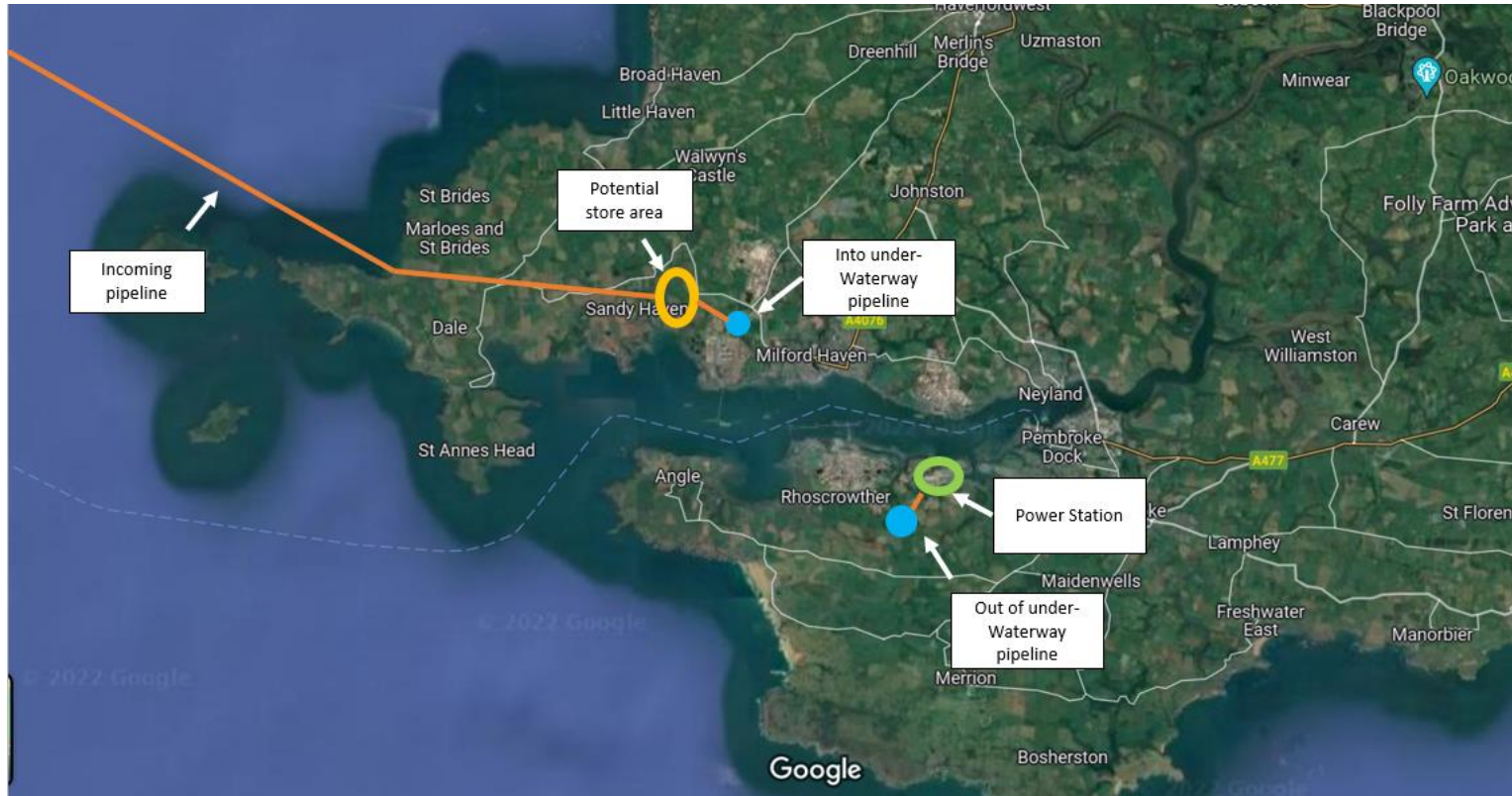
Figure A12: possible configuration for landing energy in Option 1 - bringing hydrogen onshore for storage before sending to the power station. Theoretical alternative options are to incorporate hydrogen storage into the existing LNG terminals.
