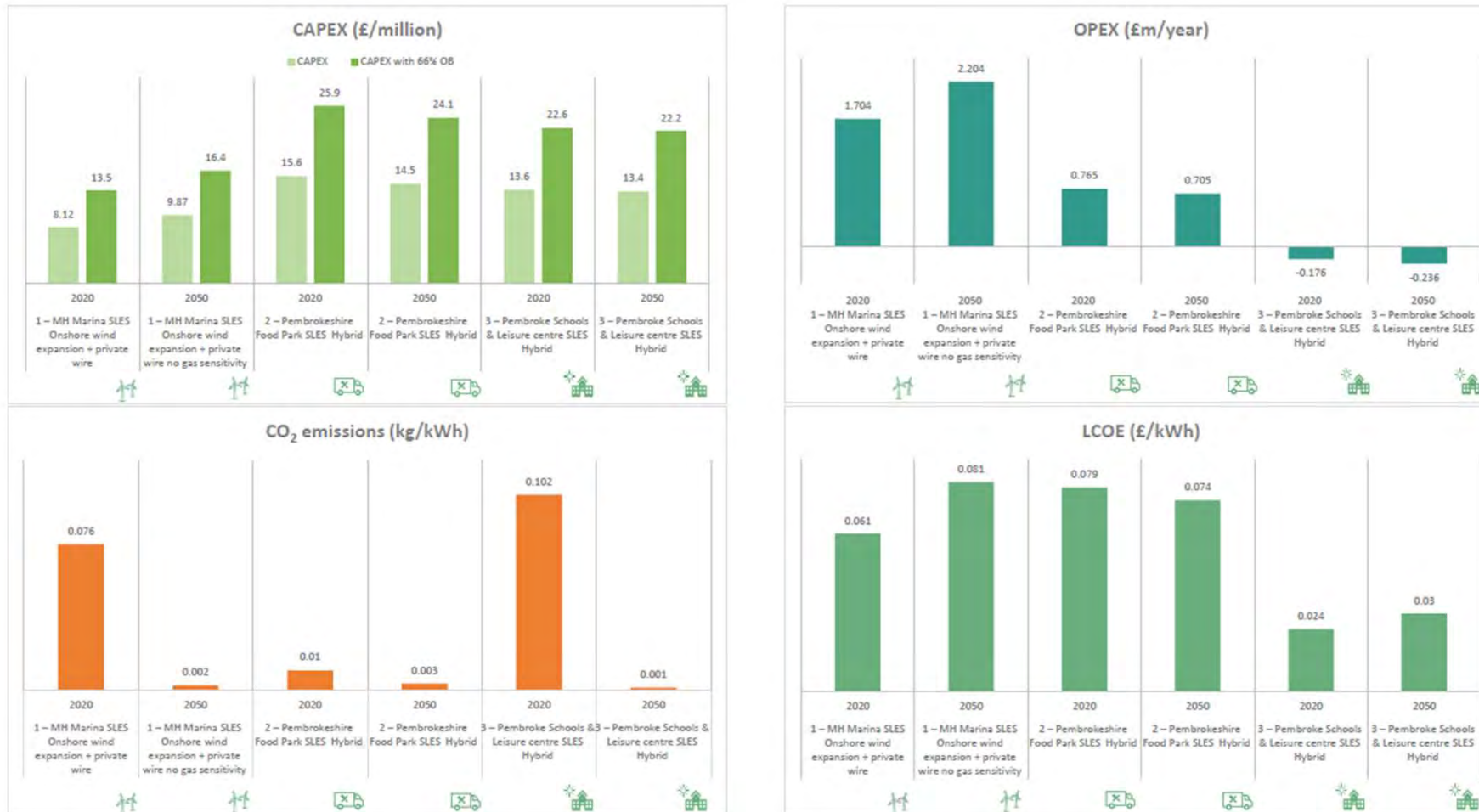
Figure 4: Graphical representation of the CAPEX, OPEX, LCOE and carbon emissions for each proposition scaled to the size / capacity of the proposition. *CO 2 emissions are shown adjusted to a 2050 view and excluding gas heating emissions in order to compare like-for-like with proposition 2 and 3.
