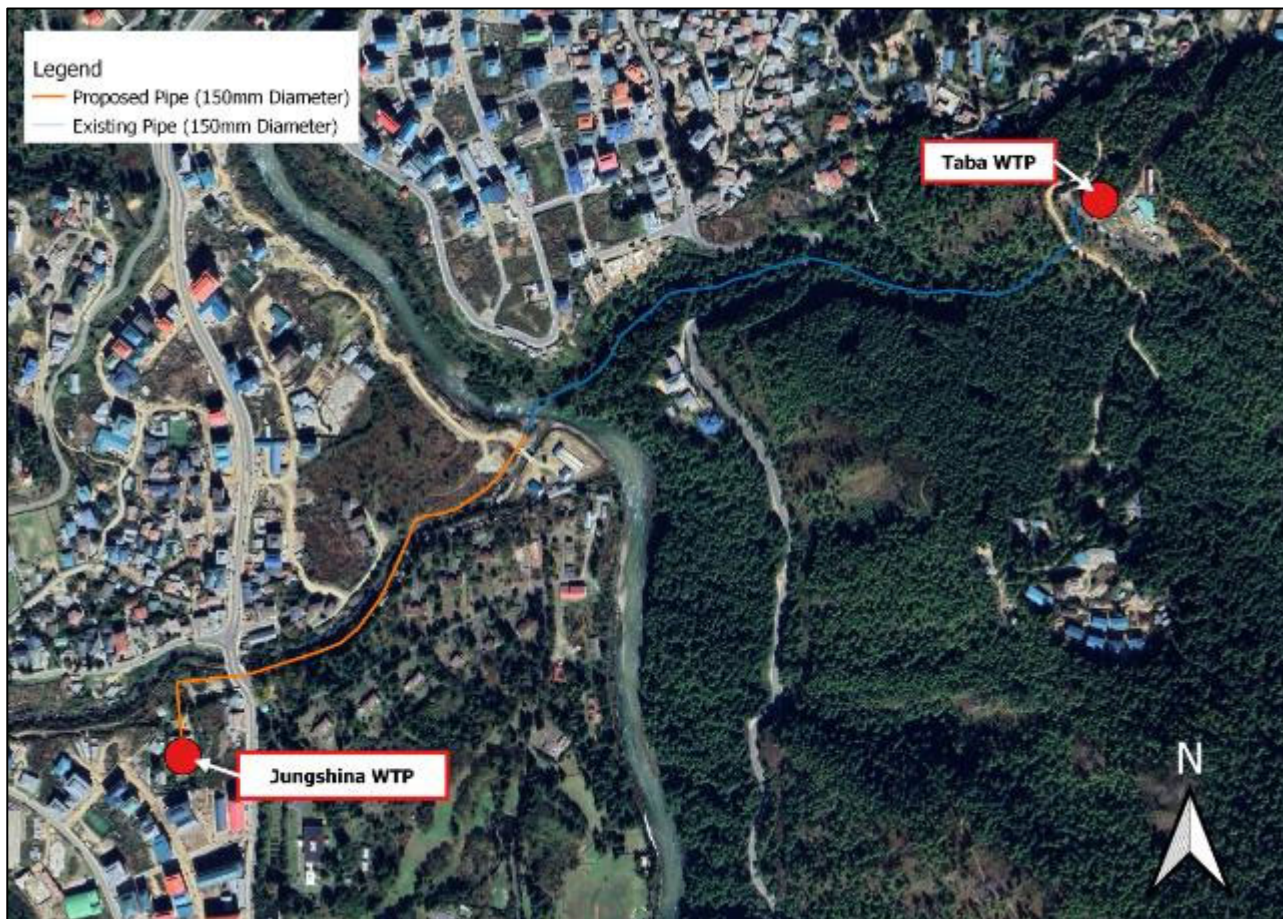
Figure 4-6: Opportunity to Reroute Raw Water from Taba Raw Water Trunk Main to Jungshina WTP
